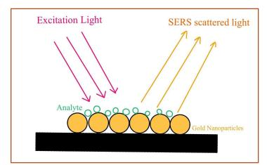
Figure 1: Raman signal enhancement through Au nanoparticles
