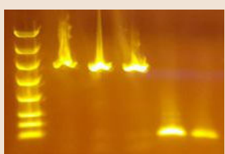
Figure 5. Our first attempt at Consensus-Degenerate Hybrid Oligonucleotide Primer (CODEHOP) design fails to amplify PBAN gene. In this experiment, we attempted to amplify the wax moth PBAN gene using the CODEHOP primers. The first well shows the 100-4,000 bp DNA markers. Wells 2-4 show the results of the silkworm PBAN primer applied to the silkworm primers, SWPBAN-FP and SWPBAN-RP (not using the CODEHOP strategy). Wells 5-6 show the results of the CODEHOP primers applied to the silkworm and wax moth DNA, respectively. The DNA from the CODEHOP wells appear to be shorter than the regular BioBrick primers on the silkworm genome used before.
