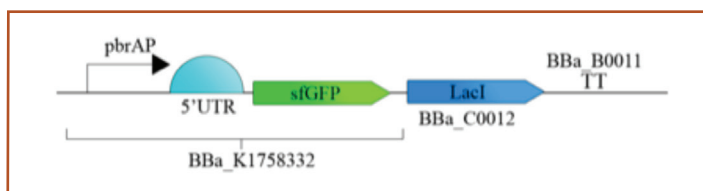
Figure 4. The above image displays the second composite part within the Renaissance lab's lead sensing system. This part produces GFP to signal the presence of lead to the user.
