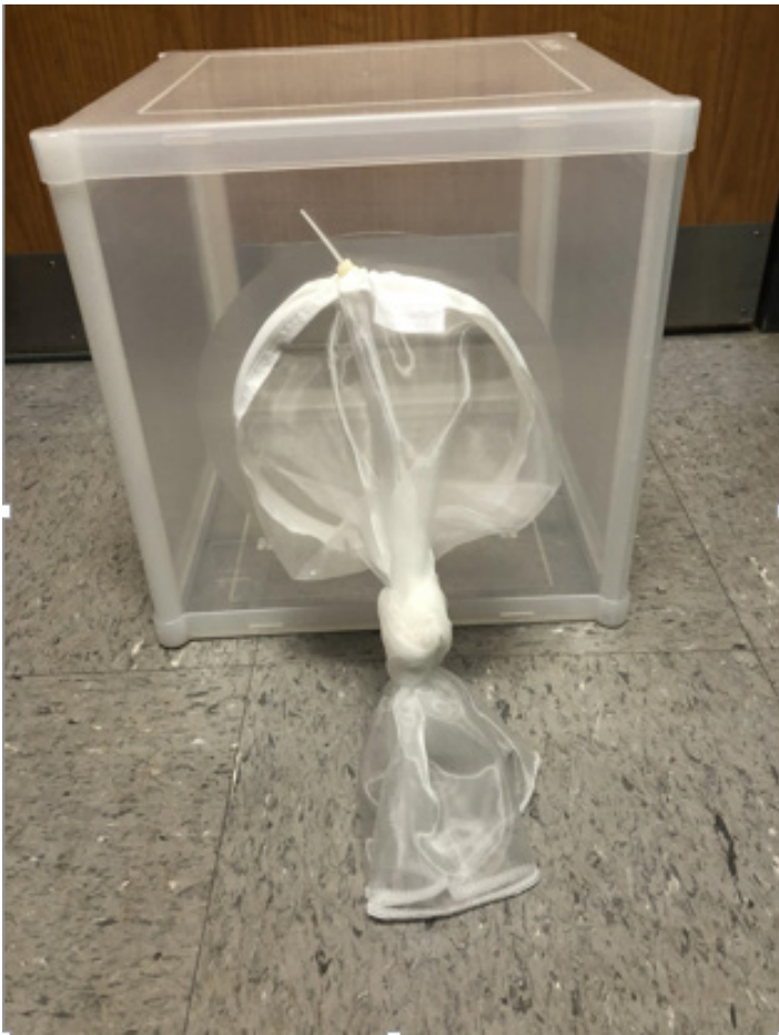
Figure 5. An 8" × 8" × 8" bug dorm was constructed and used to keep the adult A. albopictus mosquitoes in a contained area. These bug dorms also played the dual role of testing chambers in this investigation.
