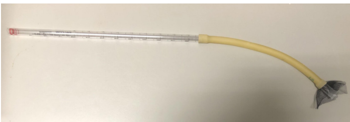
Figure 6. A homemade mosquito aspirator was assembled using a 10 mL serological pipet (left), 8" rubber tubing (middle), mosquito netting and an Eppendorf tube with the lid and bottom removed (right). Using this aspirator, adult mosquitoes could be carefully transferred to the bug dorm without the risk of inhaling the mosquito, due to the mosquito netting partition.
